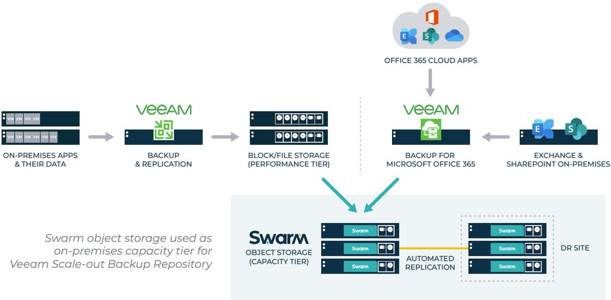
Swarm object storage used as on-premises capacity tier for Veeam Scale-out Backup Repository
